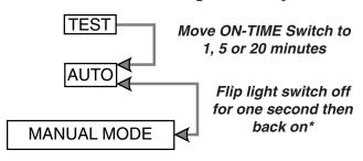
\* If you get confused while switching modes, turn the power off for one minute, then back on. After the calibration time the control will be in the AUTO mode.
